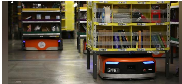
Figure 2. Kiva System Robots Operating at Amazon.
